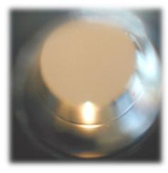
View through an inspection microscope. Clearly visible is the drawing ring in the reduction cone. The drawing die needs to be recut.
