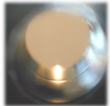
View through an inspection microscope. Clearly visible is the drawing ring in the reduction cone. The drawing die needs to be recut.
