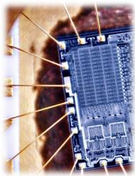
One of the most, if not the most demanding industry is the **bonding wire industry**, manufacturing gold or copper bonding wires with sizes as small as 0.010 mm, along with extremely narrow tolerances of 0.2 or even 0.1 micron.
